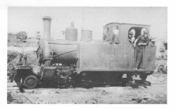
The crew of Innisfail Tramway 6 pose their charge in front of the Johnstone River. Although a Queensland Railways locomotive, the smokebox door is not of their standard pattern, but a homemade affair. Note the vital re-railing jacks on the front beam. (R.F. Ellis collection)
