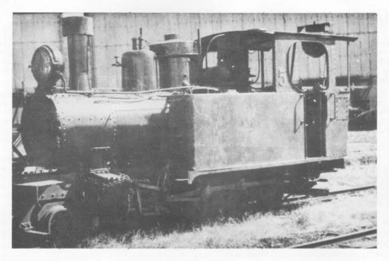
Babinda Sugar Mill No. 5 (HE 1235) was considerably altered by the addition of Queensland Railway lamps and smokebox door, extended smokebox, welded chimney with spark arrester, enlarged sand dome, extended cab roof and large vent openings in the front of the cab. (K. Rogers, G. Bond collection)
