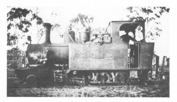
Gin Gin Sugar Mill No. 1 still carried its WDLR numberplate, in common with several other 4-6-0 tanks in Queensland. The extended smokebox, which completely spoils the locomotive's lines, is very prominent. (G. Bond)
