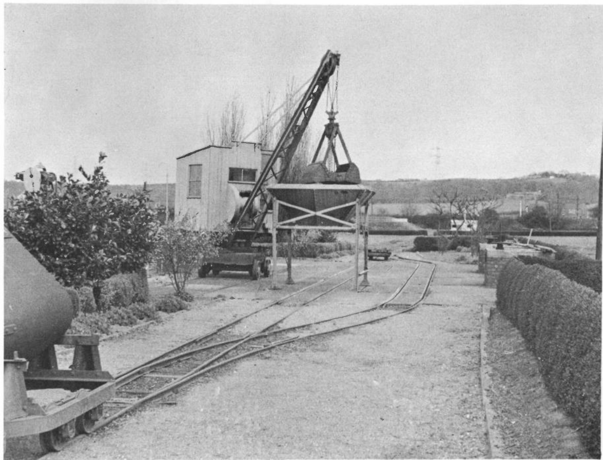
Rail mounted crane, hopper filler and section of the 2ft gauge system at Woodhouse Mill, April 1972.
