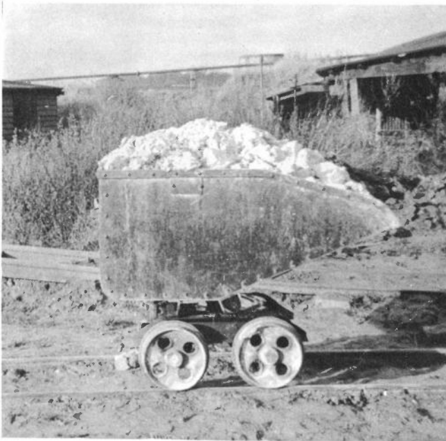
CREMER WHITING & CO. LTD, Ospringe Brickworks Oare, Faversham, Kent, 28/11/64. . . . diminutive 2ft gauge 'scoop-type' end-tip wagon loaded with clay for brickmaking. (Jim Crow)
