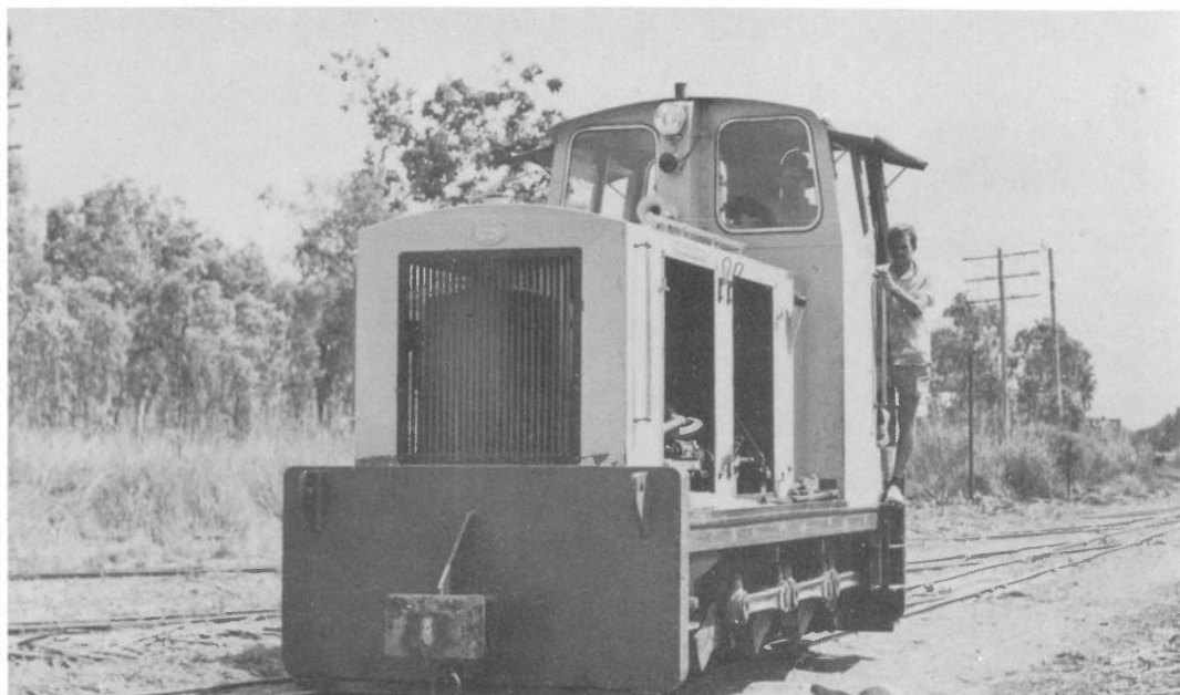
E.M. Baldwin built this 15 tonne 0-6-0DH on the frame of a Ruston Hornsby 3ft gauge 100 h.p. locomotive used by a contractor on the Snowy Mountains Hydro-electric scheme. In September 1968 it was photographed at Plane Tree Mill, their No.9. (John Armstrong)
