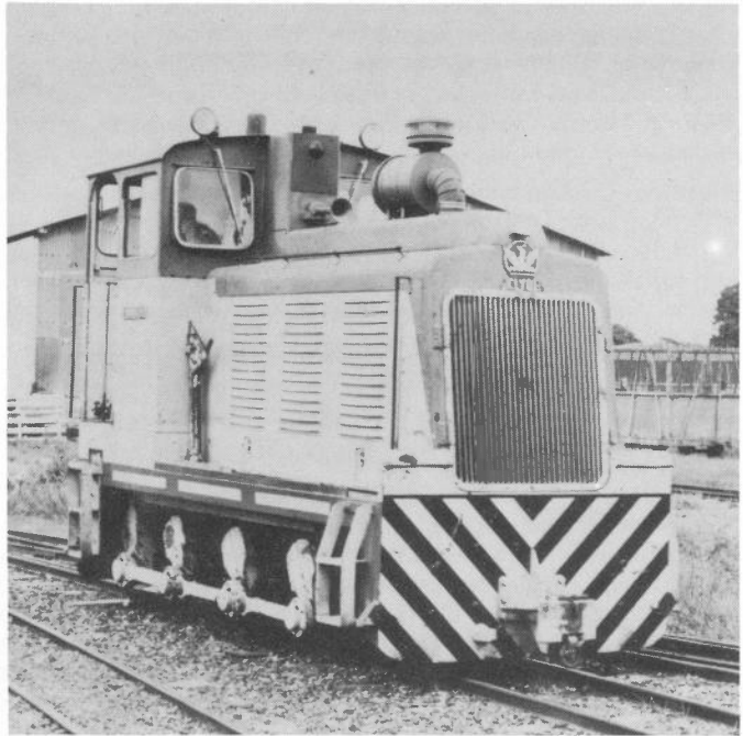
HOME BUSH, an early Clyde model DHI-71 0-6-0DH built in 1955, seen here at Racecourse Mill in September 1978. The large air filter is a recent addition. (B.J. Webber)
