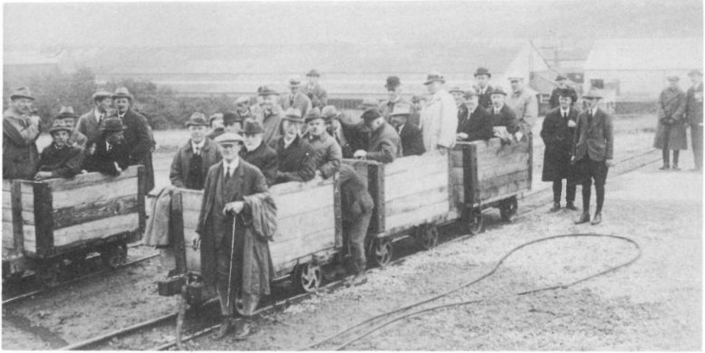
The foot of Dolgarrog incline, probably in the early 1920's, with a party about to set off on an outing to Llyn Cowlyd. The haulage cable is already attached to the leading wagon, whose occupants seem unmoved by the experience in prospect. (collection J.M. Ryan)
