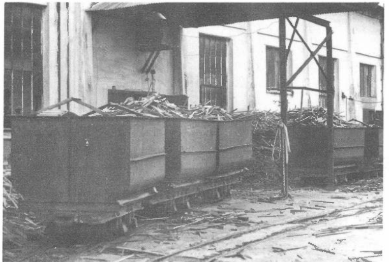
These wagons are fitted with unusual "clamshell" bodies which can be lifted from the frame, and opened to discharge the load into the boiler house. (R.A. Bowen)
