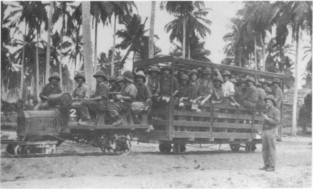
Ford lorry 2, which also carries K 1664 below the running number, with a passenger trailer on one of the 60cm gauge lines. A similar picture shows Ford 4, lettered "Sergeants Only", with an open trailer. (collection G Richardson)
