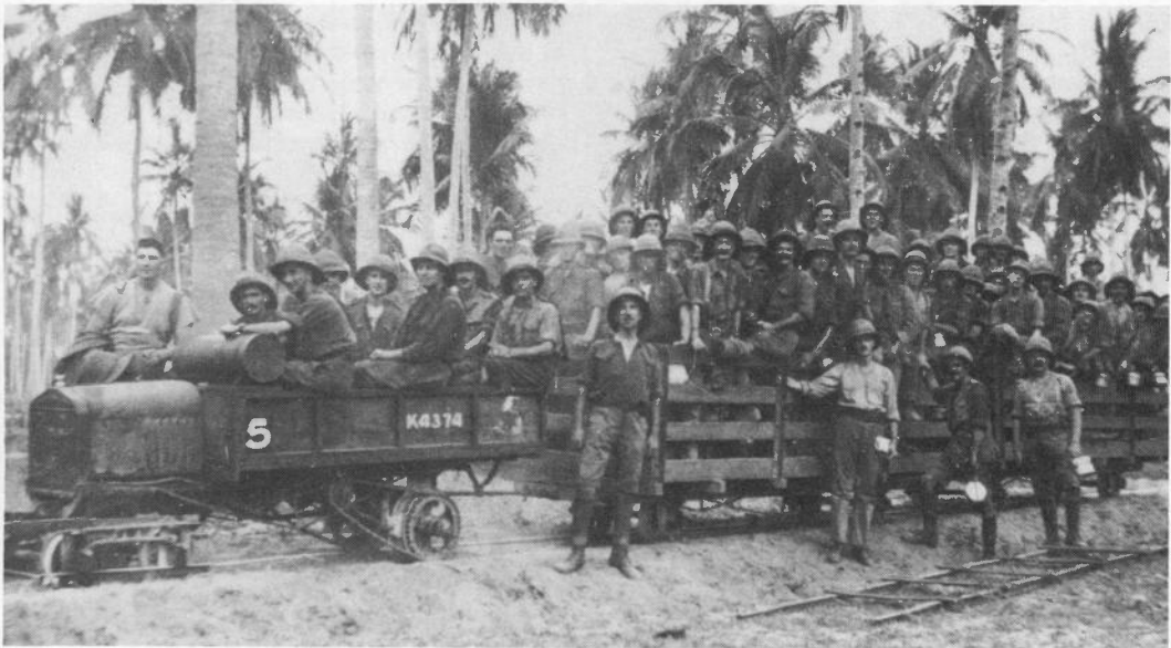
Ford 5 at Kilwa or Lindi. This differs in several details from the tractor above, and has a black radiator shell with a separate core, introduced in 1916, rather than the earlier brass radiator. (collection G. Richardson)
