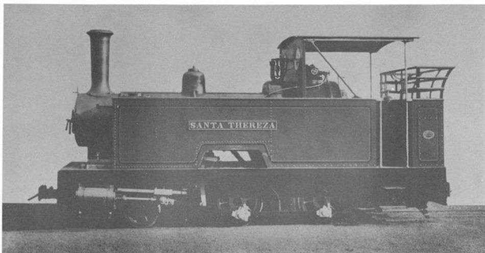
SANTA THEREZA, one of the largest of the 2-4-0 tanks, had a raised, circular firebox, extended side tanks, and Bagnall-Price valve gear. (collection A.C. Baker / T.D.A. Civil)
