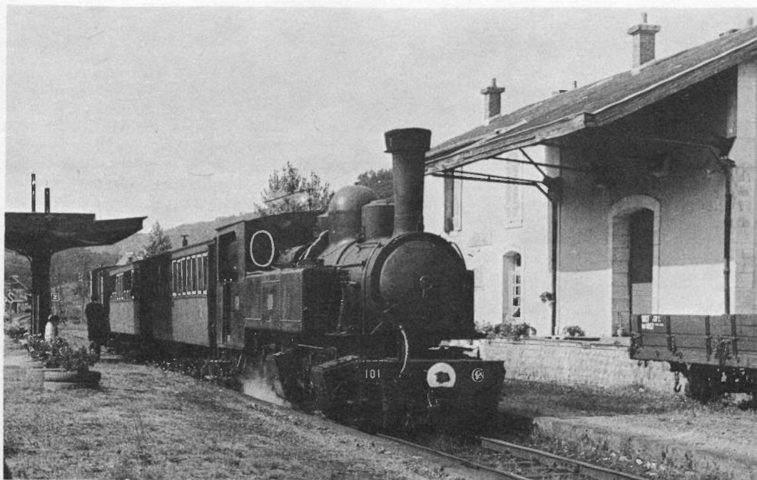
P.O. Correze (France). Forges station on the Argentat line, with Blanc Misseron 0-4-4-0T Mallet No 10L and special train, 30th August 1969. Both the locomotive and the coaches have since been preserved. (V.W. Blake-Dyke).
