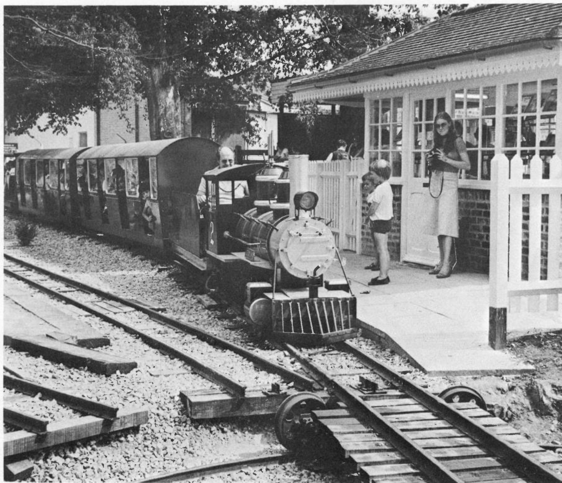
Severn-Lamb 'Rio Grande' class 15in gauge 1-8-0 in use at Longleat in July 1976. Severn -Lamb Ltd. have built a number of these internal combustion engined locos in both 10 1/4in and 15in gauges over the last few years. (Robin Butterell).
