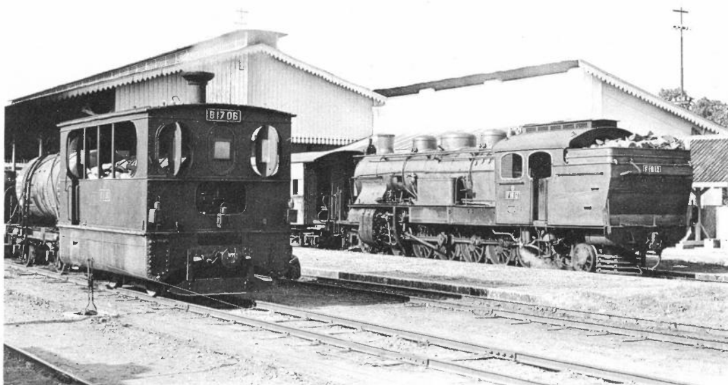
INDONESIA — 3ft 6in gauge contrasts at Kepiri Station, Java on the PNKA Wood burning 2-12-2T F10.12 and 0-4-0 steam tram B17.06 in October 1973. (L.A. Nixon).
