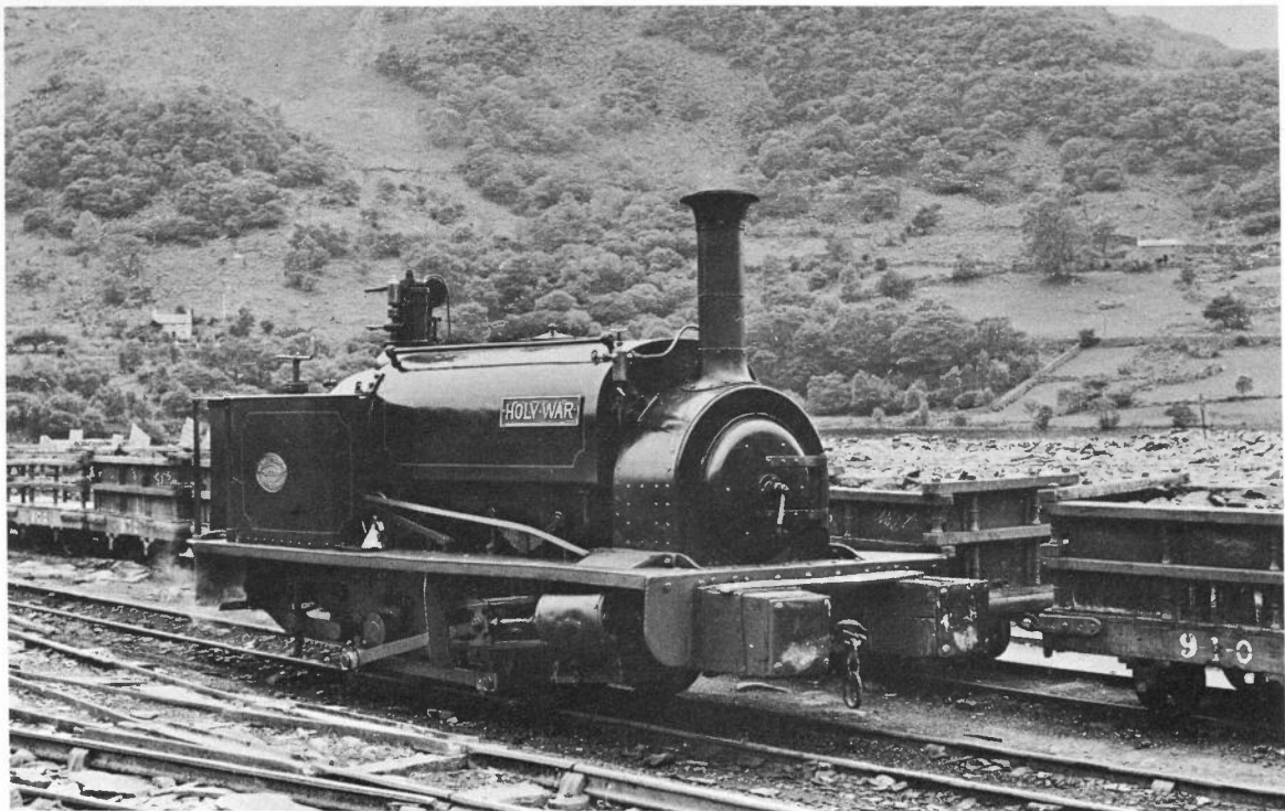
The Hunslet slate quarry saddletanks were probably the most well-known industrial narrow gauge steam locos in Britain. The last one to remain in active industrial service was HOLY WAR at Dinorwic, which finally ceased work late in October 1967, although this particular picture was taken eleven years earlier. (Ivo Peters).
