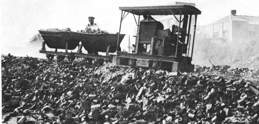
Industrial narrow gauge railways have been used in a wide variety of locations. Surely one of the most unsavoury was the 1ft. 8in. gauge system at the Royal Borough of Kensington's Wood Lane destructor works, where Lister petrol loco 40011 is seen propelling two loaded skips up the steaming rubbish tip on 26th. August, 1954. Note that the loco has been rebuilt with the engine of a Scammell lorry. (Frank Jux).
