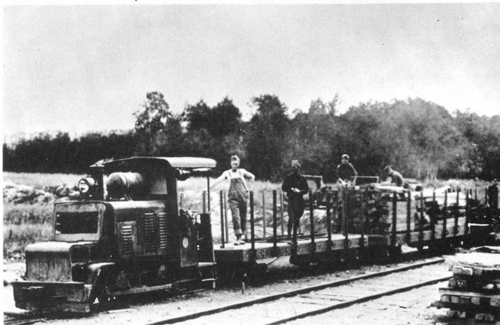
Bwn 0-4-0PM on active service in France in 1918 with the USATC (Ron Redman collection)
