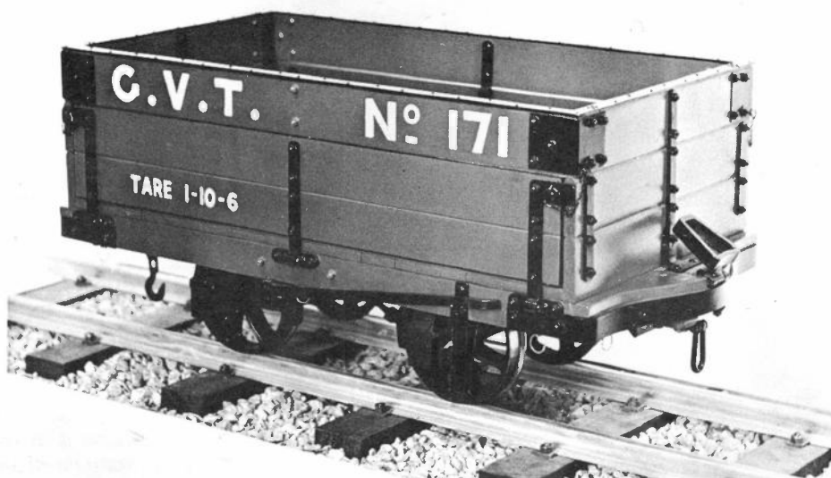
1) Model of Glyn Valley Tramway open granite wagon as constructed by the Midland Railway Carriage & Wagon Co. Ltd in c1888 for the Glyn Valley Tramway Company. Scale 1½in to 1ft.
