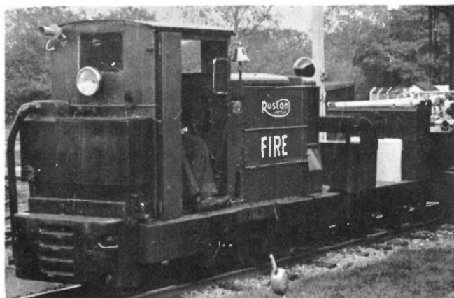
No.194784 (44/48HP). A rarely seen and very rarely photographed loco. AMW165 is kept in permanent readiness on the fire-fighting train at M.O.D. Dinton Depot, Wilts and is painted in 'fire — engine red' with white lettering. Like all Rustons owned by the Ministry it is fitted with flame-proofing equipment at the rear (H. T. Caffyns)
