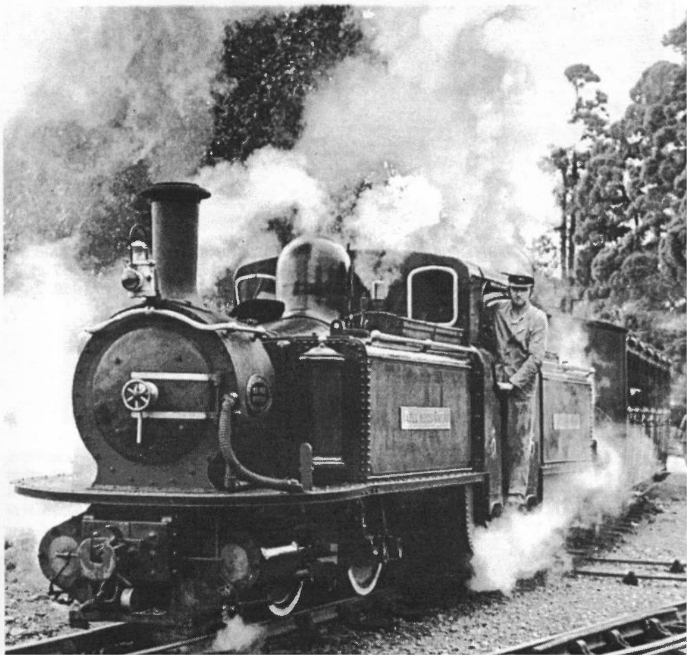
2nd Place - Category A (Narrow Gauge Steam) By: Mr. P. J. Shoesmith of Birmingham. Photo: Festiniog Railway 1ft 11½in gauge, in N. Wales. EARL OF MERIONETH/IARLL MEIRIONYDD 0-4-4-0T Fairlie (built by the FR in 1885) at Tan-y-Bwlch on a Portmadoc to Dduallt train, 23rd August 1970.
