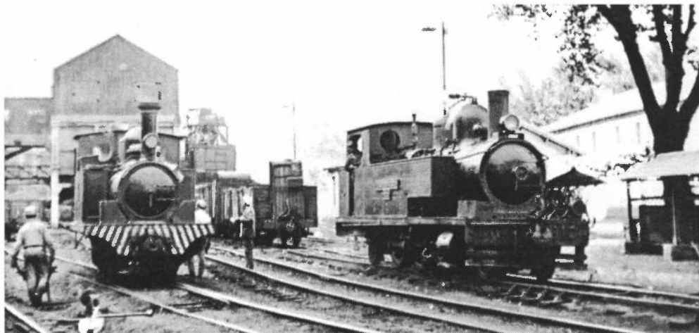
Hulleras de Sabero y Anexas (Metre gauge) No. 10, EL ESLA (Sharp Stewart 3343 of 1885) 0-6-0T, and No. 13 VALDERRVEDA (Sharp Stewart 4018 of 1894) 2-6-2T (the latter on hire from Ferrocarril de la Robla). Sabero Screens in September 1967. (Ron Cox)
