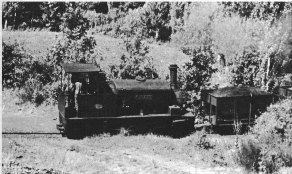
Vasco-Leonesa S.A. (550mm gauge) SANTAANA, 0-4-2ST (Hudswell Clarke 640 of 1903) drifting downhill with a train of loaded coal hoppers, September 1970.
