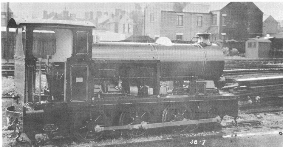
No.3014. Outside Baguleys Uxbridge Street Works in pouring rain, 1938. This unique 0-6-0 Petrol machine was the third loco built for the Trentham Gardens line. (Engine covers removed for this Makers photograph of DUNROBIN).
