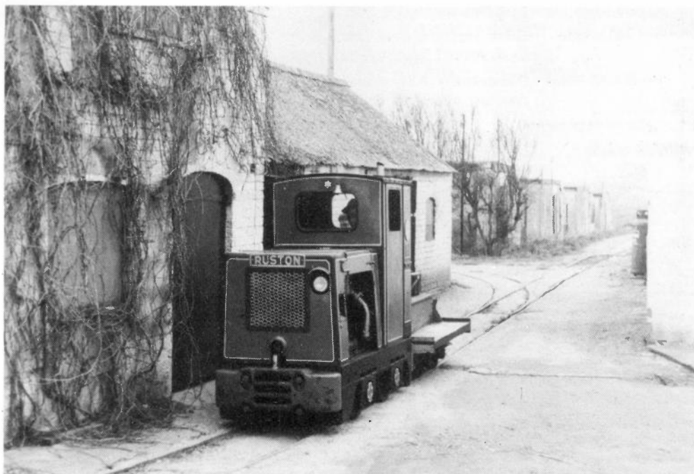
RH 371937 trundles through the front yard en route to the locomotive shed. The track on which it is standing is the original, together with the point and line curving left. The main line runs straight on. (D. Billmore)
